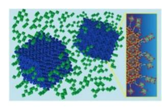
Nanocrystals of indium tin oxide (shown here in blue) embedded in a glassy matrix of niobium oxide (green) form a composite material that can switch between NIR-transmitting and NIR-blocking states with a small jolt of electricity. A synergistic interaction in the region where glassy matrix meets nanocrystal increases the potency of the electrochromic effect.
